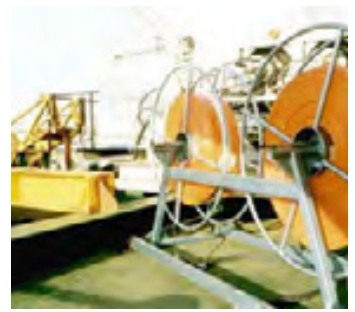
SeaSerpent DRS system positioned on deck at aft overboarding station.
