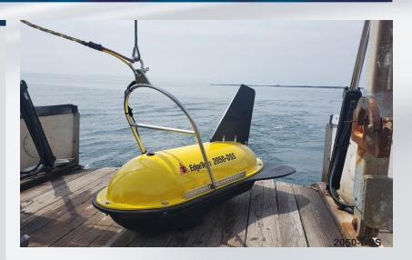
The EdgeTech 2050-DSS is the latest product to combine EdgeTech's highly successful line of side scan sonars and sub-bottom profilers into one fully integrated system. This is especially useful where high resolution sub-bottom profiler data, that requires the system to be towed near the seabed, is required.
